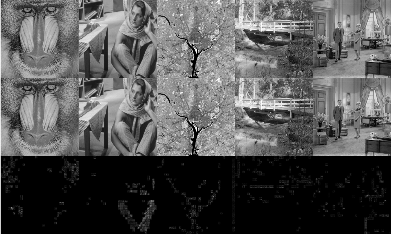
Fig. 9. Original, watermarked and difference images using the proposed method: Baboon , Barbara , Map , Bridge , and Couple . For each image, the top one is the original test image, the middle one is the watermarked image, and the bottom one is the five times scaled of the absolute difference between the watermarked and the original image.
