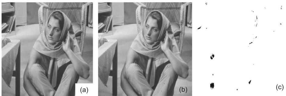
Fig. 19 a Host image Barbara b Watermarked image Barbara c Error image between host and watermarked image
