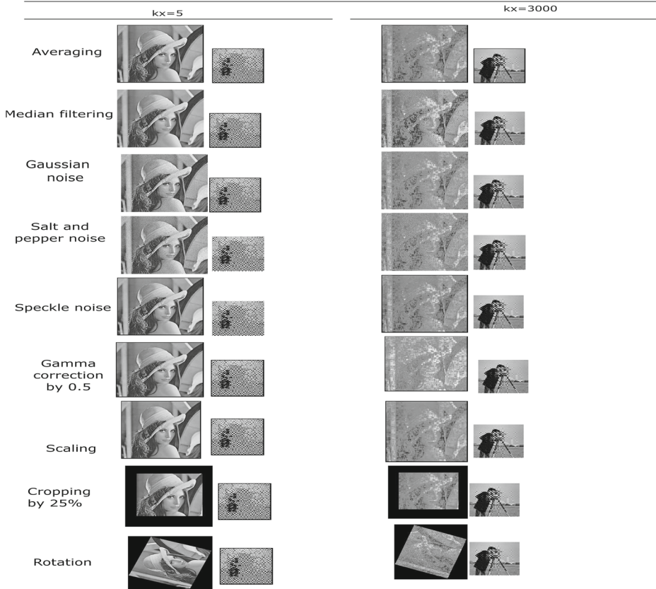
Fig. 21 Effect of single scaling factor kx on imperceptibility and robustness in [7]
