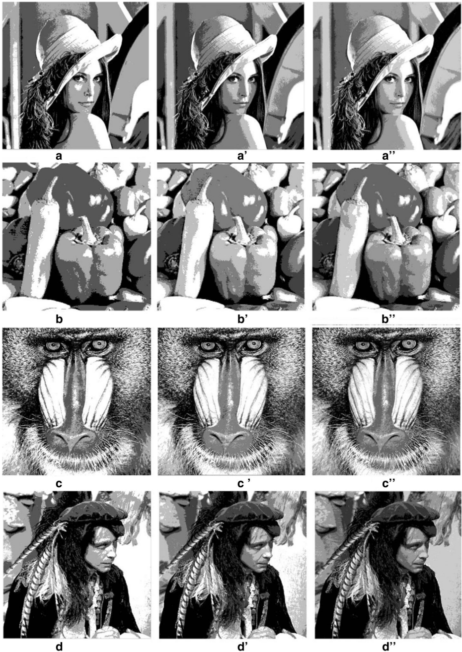
Fig. 5 Thresholded images obtained by the hybrid method on Kapur thresholding (a)–(j) represents 3-level thresholding, (a')–(j') represents 4-level thresholding, (a'')–(j'') represents 5-level thresholding
