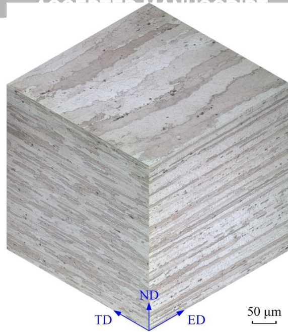
Fig. 2. Three-dimensional optical micrograph of the AA2195 extruded plate.
