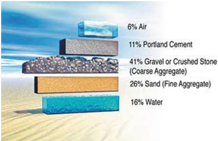
Fig. 1.1 Constituents of concrete
