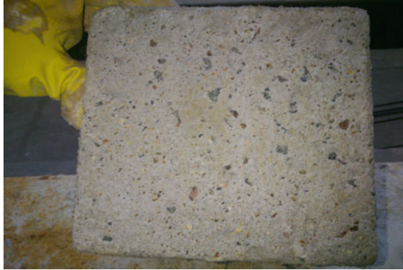
Fig. 5.5 Specimen of normal concrete immersed in 5% H_2SO_4
