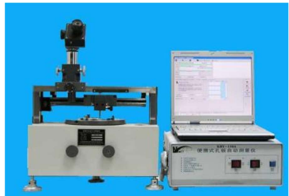
Fig. 4. The HXJ – 150 A portable orifice automatic measuring instrument.
