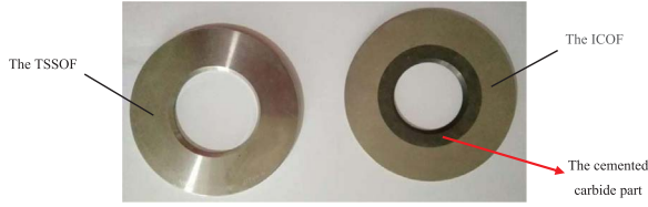
Fig. 2. Two kinds of orifice flowmeters: the TSSOF and the ICOF.
